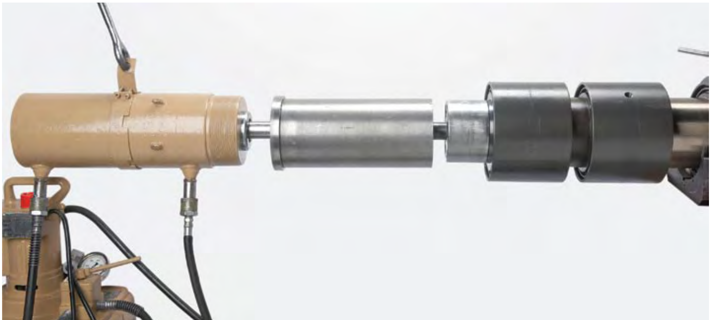
Fig. 28 Tooling used to push bearing onto shaft
