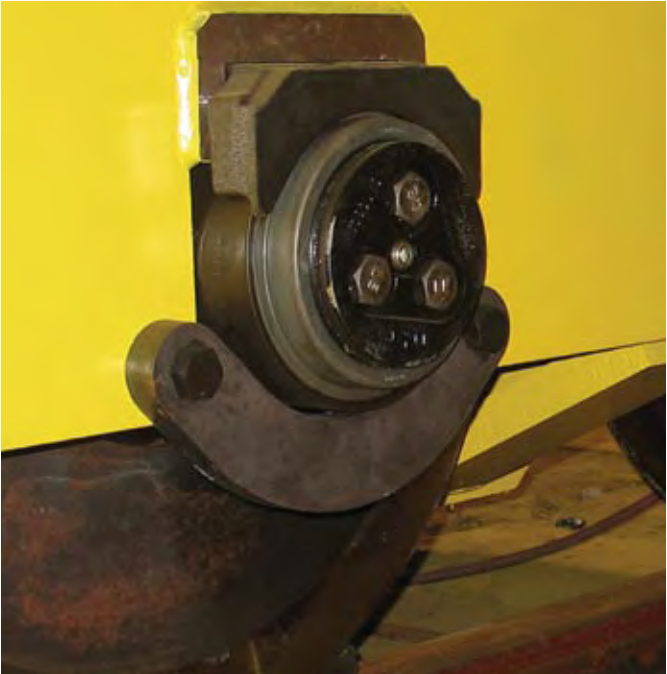
Fig. 8 Narrow adapter mounting on trolley safety bar
