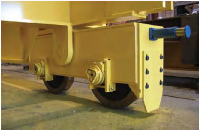
Fig. 5 Standard end cap design
