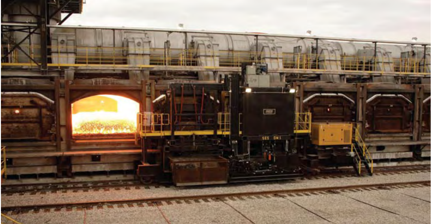
Fig. 20 Coke transfer car equipped with AP bearings
