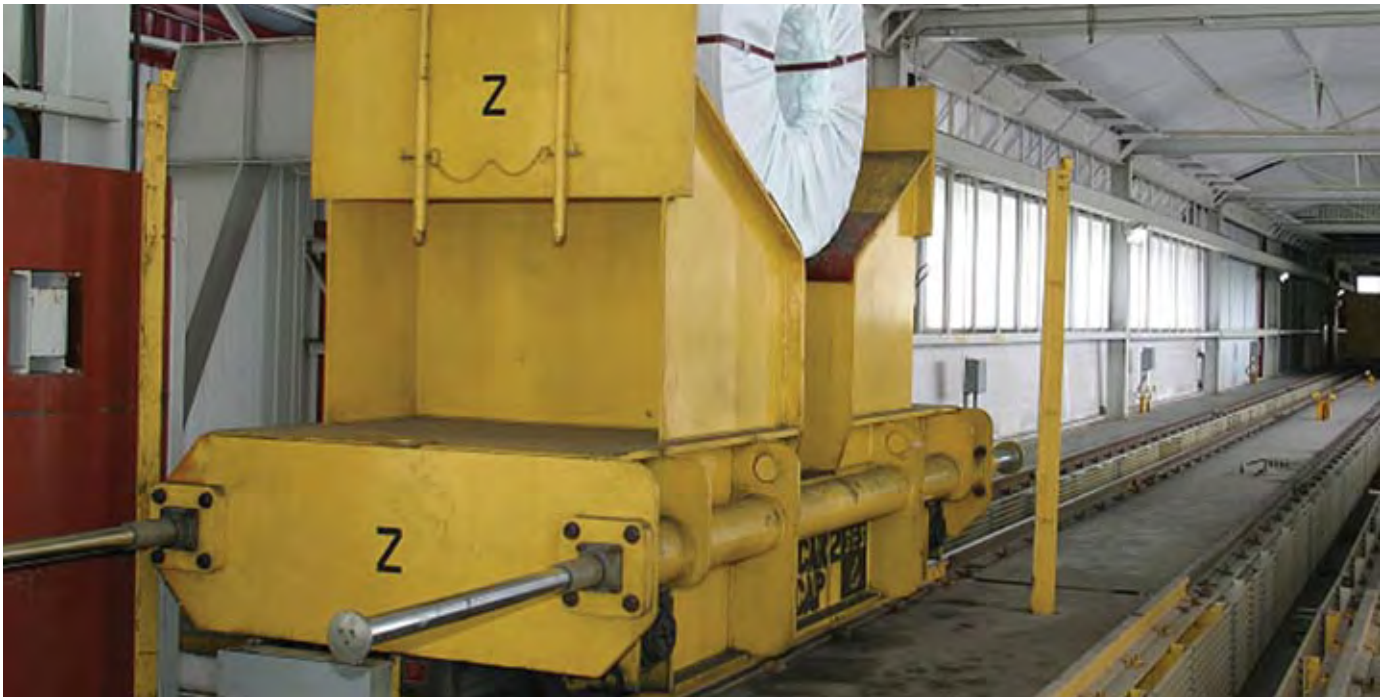
Fig. 18 Coil transfer car equipped with AP bearings on axles
