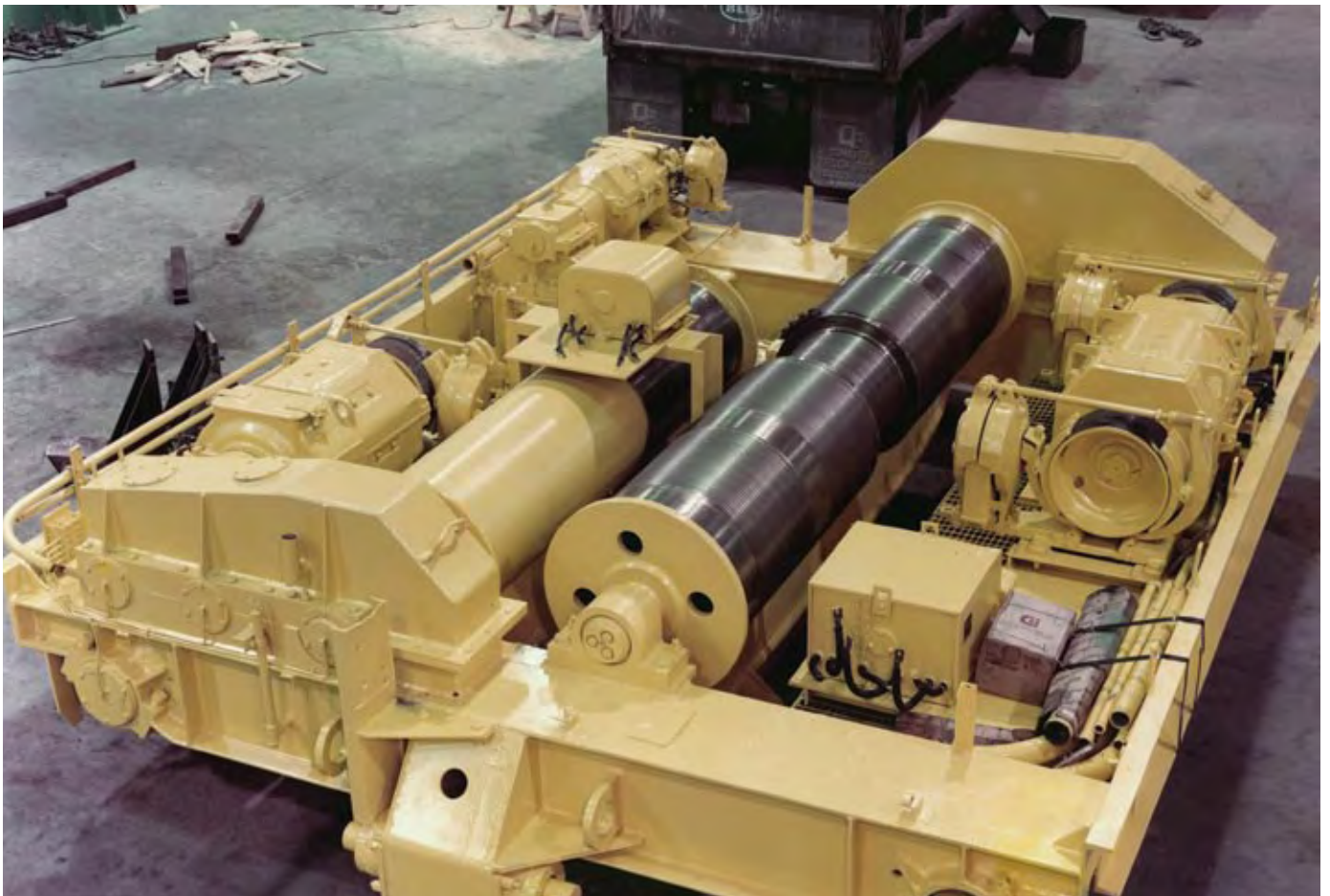
Fig. 6 Trolley utilizing AP bearings with recessed end cap for wheel and drum drive
