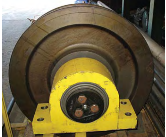
Fig. 12 AP bearings used in pillow block application
